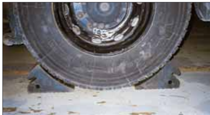
Correct use of Trailer Chocks when stowed athwartship and on ramps.
